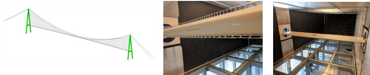
Figure 2: Left: finite element model; middle: close-up photo of a section model with barriers and guide vanes; right: entire section model in the wind tunnel.
